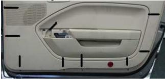
9. Lift up on the interior panel, removing it from the door. Remove any remaining electrical connections.
