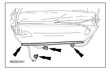
10. Release the pin-type retainer and backrest trim from the backrest frame.
