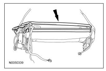
9. Release the inner J-strip at the bottom of the backrest trim cover and remove the harness wires from the backrest cover.
