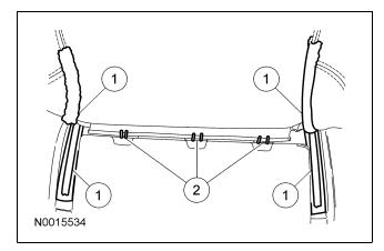
12. A WARNING: To correctly retain the backrest trim cover and allow correct deployment of the seat side air bag module, make sure to install 2 hog rings to attach the backrest trim cover wire to the listing wire in each foam pad window. Failure to follow this instruction may result in personal injury in the event of a seat side air bag module deployment.
