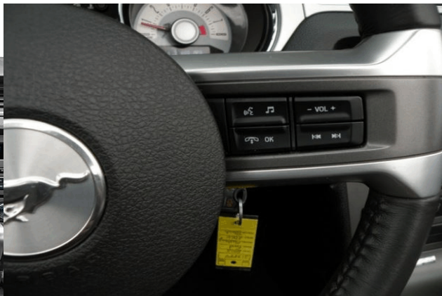
#SW6714 Used with SYNC & Shaker radio heads. Not used with Navigation. Note audio controls. Note: "ok" button on the switch.
