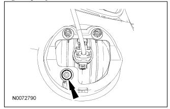
1. **NOTE:** Horizontal aim is not required for this vehicle and is not adjustable. Consult your state vehicle inspection center for recommended tolerance ranges for visual aiming.
