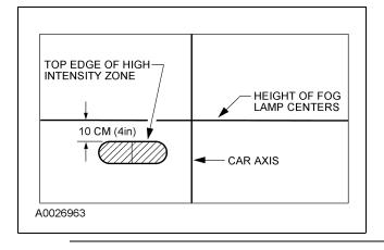
4. If necessary, rotate the adjusting screw until the fog lamp beam is within specification.
