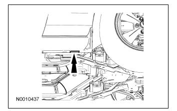
To jack the front end, lift at the pinch welds located at the front opening of the rocker panels.
