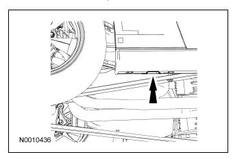
To jack the rear end, lift at the pinch welds located at the rear opening of the rocker panels.
