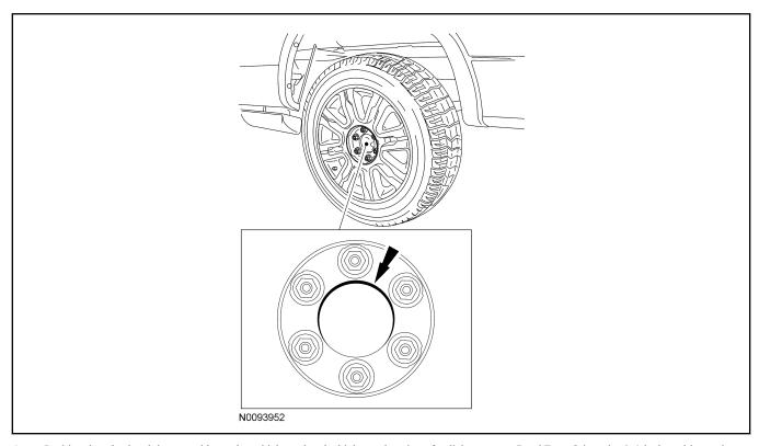
1. Position the wheel and tire assembly on the vehicle so that the high spot location of radial run-out or Road Force® is at the 6 o'clock position and install the wheel nuts by hand until snug.
