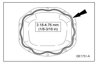
3. **NOTE:** The differential housing cover must be installed within 15 minutes of application of the silicone sealant, or new sealant must be applied. If possible, allow one hour before filling the axle housing with axle lubricant to make sure the silicone sealant has cured.
