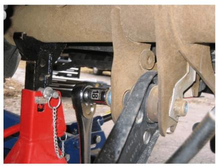
Remove the clip off the ebrake cable and disconnect the he cable (refer to the pdf, my picture didn't come out)Using an 18mm socket wrench, disconnect the front of the LCA arm, then disconnect the back
