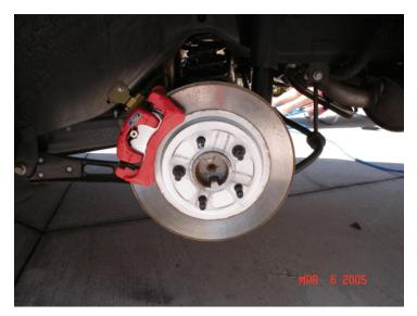
Next, use a flat blade screwdriver to pry up on the e-brake cable and pop it out of it's retainer
