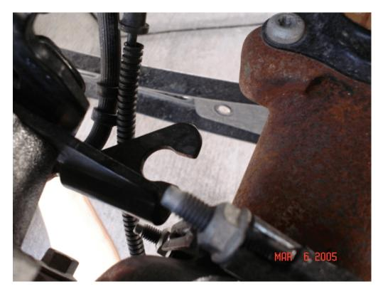
Use an 18mm socket to remove the bolt at the front of the LCA, then switch to a wrench when you run out of room - you'll know what I'm talking about when you do it
