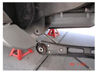
Use the 18mm socket again to remove the rear bolt, and the LCA will slip out of place
