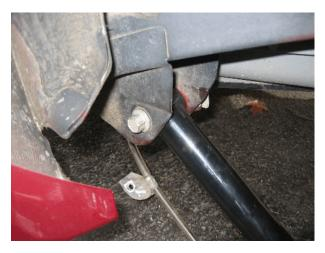
ONLY DO ONE ARM AT A TIME. IF YOU DISCONNECT BOTH AT THE SAME TIME YOUR AXLE WILL SHIFT WAY OUT OF POSITION!!!!Now would be a good time to put thick lithium grease inside the steel bushings on the BMR arms. Don't use regular grease because it will dry up the poly bushings over time. This might prevent squeeking down the road. I actually bought grease to do this
