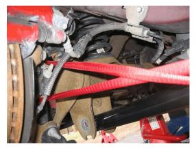
Now your strap is in position and ready to shift back into place Tighten the ratchet until the holes in the rear bracket line up with the LCA Insert the bolts and tighten all the way with a torque wrench to 129 lb-ft (1550 in/lb). That is Ford's factory spec. There were no instructions with the BMR arms. A lot of people here are saying to torque them to 75 lb-ft, that is not tight enough, I suspect this is what is causing some of their noise problems
