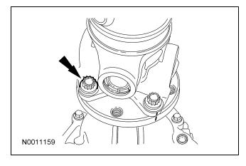
5. CAUTION: The driveshaft flanges fit tightly on the transmission flange pilot. Never hammer on the driveshaft or any of its components to disconnect the driveshaft flange from the transmission flange pilot. Pry only in the area shown, with a suitable tool, to disconnect the driveshaft flange from the transmission flange pilot.
