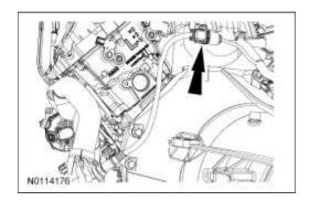
10. Remove the bolt and position the steering intermediate shaft aside.
