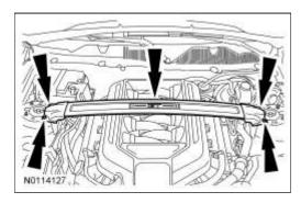
6. **NOTE:** The engine appearance cover rubber grommets may remain on the cover. If so, remove the grommets from the cover and install them on the intake manifold before installing the cover.
