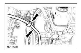
20. If equipped, detach the Evaporative Emission (EVAP) tube from the LH valve cover and the LH inner fender.
