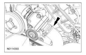
25. Disconnect the 2 heater hose quick connect couplings from the heater core. For additional information, refer to Section 412-00.
