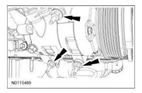
51. Remove the 2 separator plate bolts.
