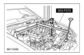
44. Detach the wiring harness retainers from the RH side of the oil pan and the RH engine support insulator bracket stud bolt.
