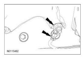
47. **NOTE:** The RH engine support insulator has been removed from the graphic for clarity. Remove the 2 bolts, the 2 stud bolts and the RH engine support insulator bracket.
