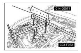
56. NOTICE: Do not support the transmission by the fluid pan, failure to follow this instruction may result in serious damage to the transmission.
