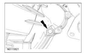
54. Loosely install the 3 underbody shield bolts.
