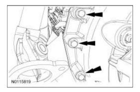
53. Remove RH transmission-to-engine bolt.
