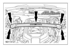
11. **NOTE:** The engine appearance cover rubber grommets may remain on the cover. If so, remove the grommets from the cover and install them on the intake manifold before installing the cover.
