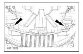
52. Remove 3 LH transmission-to-engine bolts.
