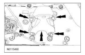
50. Remove the 3 stud bolts and position the A/C compressor aside.
