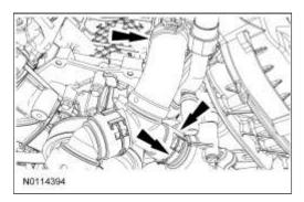
24. Disconnect the lower radiator hose from the engine.
