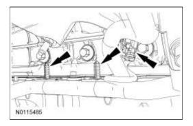
45. Detach the wiring harness retainers from A/C compressor stud bolt and the RH side of the oil pan.
