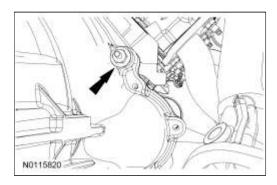
58. Using the Engine Crane, separate the engine from the transmission and remove the engine from the vehicle.
