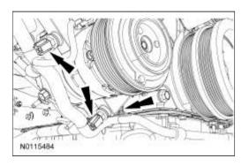
46. Remove the nut and ground strap from the RH engine support insulator bracket.
