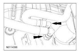
26. Disconnect the engine cooling fan electrical connector.
