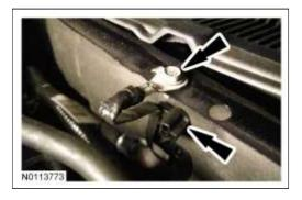
14. **NOTE:** It is not necessary to separate the Air Cleaner (ACL) outlet pipe and the <u>ACL</u>, the 2 components can be removed as an assembly.
