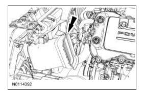
23. Remove the spring clip, the clamp and disconnect the coolant bypass T assembly from the engine.
