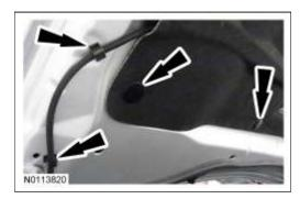
8. Detach the 2 windshield washer hose retainers and disconnect the 2 windshield washer hose C-Lock Couplers. For additional information, refer to <a href="Section 501-16">Section 501-16</a>.
