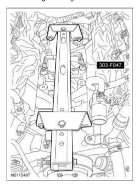
41. NOTICE: Do not position the legs of the Engine Support Bar on the fenders. Instead, the legs should be positioned on the body structure near the suspension structioner. Failure to follow these instructions may result in body damage.
