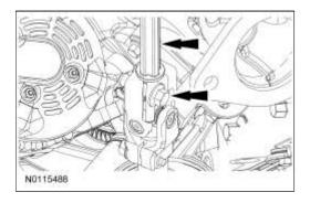
49. **NOTE:** The LH engine support insulator has been removed from the graphic for clarity. Remove the 3 bolts, the stud bolt and the LH engine support insulator bracket.
