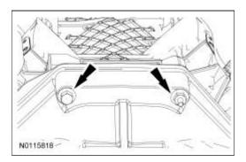
40. Install the Engine Lifting Bracket.
