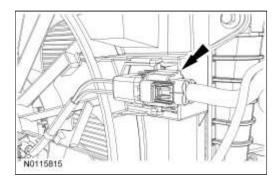
27. Remove the bolt, the stud bolt and the engine cooling fan assembly.
