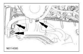
36. Disconnect the middle PCM electrical connector, the 16 pin electrical connector and detach the wiring harness retainers from the PCM bracket.
