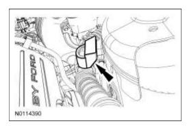
16. Remove the 8 pin-type retainers and the upper radiator sight shield.
