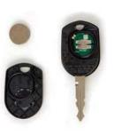
Use CR2032 Battery Replace with + side up. Do not wipe battery terminals.
