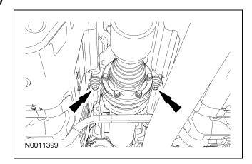
CAUTION: If new driveshaft flange bolts are not available, coat the threads of the original driveshaft flange bolts with Medium Strength Threadlocker TA-25 meeting Ford specification WSK-M2G351-A5.
