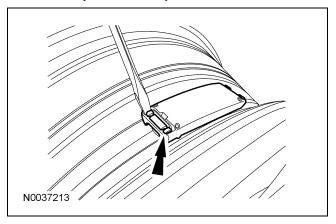
3. **CAUTION:** Do not use a large screwdriver. Apply minimum force during removal or damage to the sensor may occur.
