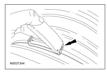
NOTE: The locking clip can only be fully seated when installed in the correct orientation. If the sensor locking clip cannot be fully inserted, then the sensor may not be fully seated on the cradle or the locking clip may be inserted backward.
