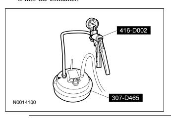
16. Allow the fluid to drain. Make sure that the fluid temperature is between 27°-49°C (80°-120°F). When the fluid comes out as a thin stream or drip, the fluid is at the correct level.
