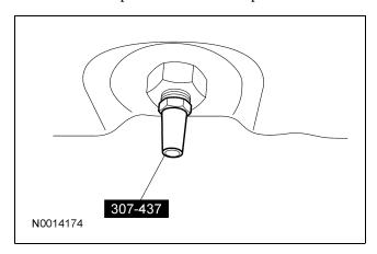
9. **NOTE:** Prior to filling the special tool with clean transmission fluid, make sure that the canister is clean.
