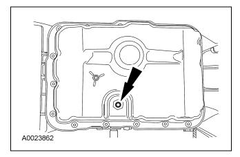
8. Install the special tool into the pan.
