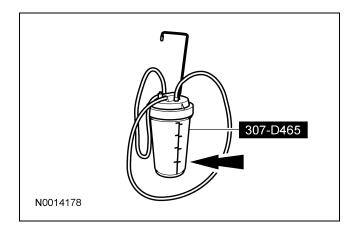
10. Hang the special tool under the vehicle. Position it upright and close to the transmission.
