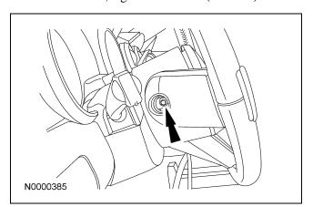
4. Disconnect the 2 driver air bag module electrical connectors.
