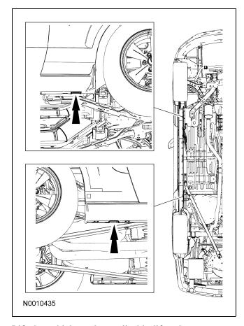
Lift the vehicle at the applicable lift points.
