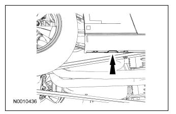
To jack the rear end, lift at the pinch welds, located at the rear opening of the rocker panels.
