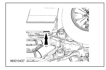
To jack the front end, lift at the pinch welds, located at the front opening of the rocker panels.
