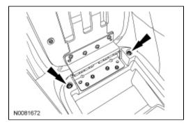
9. Remove the floor console finish panel.
