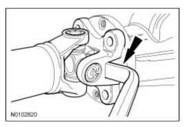
6. **NOTE:** The center bearing spacers must be installed between the body and the center bearing bracket.
