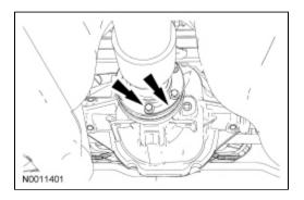
4. NOTE: If new driveshaft flange bolts are not available, coat the threads of the original driveshaft flange bolts with threadlock and sealer.
