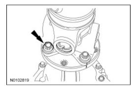
5. **NOTE:** The driveshaft flanges fit tightly on the transmission flange pilot. Never hammer on the driveshaft or any of its components to disconnect the driveshaft flange from the transmission flange pilot. Pry only in the area shown, with a suitable tool, to disconnect the driveshaft flange from the transmission flange pilot.
