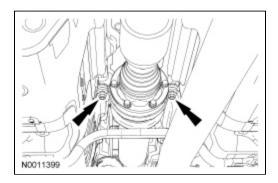
7. **NOTE:** The driveshaft flanges fit tightly on the transmission output flange pilot. To make sure that the driveshaft flange seats squarely on the transmission output flange, tighten the driveshaft flange bolts evenly in a cross pattern.
