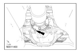
3. Remove and discard the 6 driveshaft CV joint bolts and CV joint washers, then disconnect the CV joint from the pinion flange.
