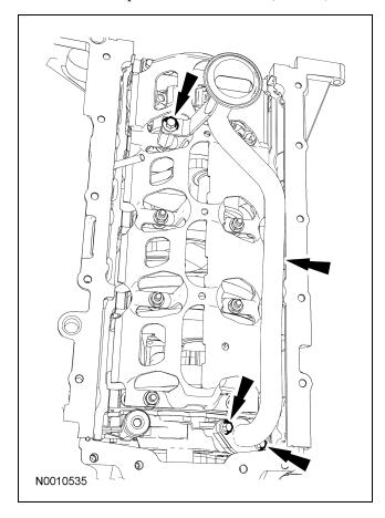
Install the oil pan. For additional information, refer to Engine Lubrication Components — Exploded View and Oil Pan in this section.
