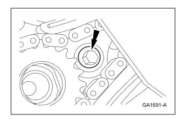
33. Position the jackshaft sprocket and chain.
