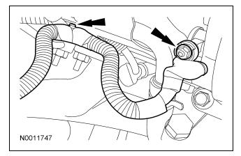
132. Connect the generator and throttle body electrical connectors.
