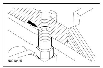
59. Install new seals on the 2 silver bolts and loosely install them in the cylinder block cradle.
