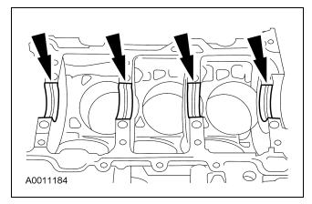
3. **NOTE:** The crankshaft main bearings are precision selective fit. Inspect the bearing clearance. For additional information, refer to Section 303-00.
