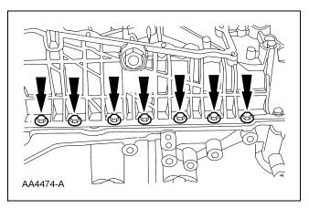
54. Install and hand-tighten the bolts.
