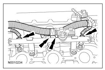
114. Connect the 3 LH fuel injector electrical connectors and attach the wiring retainer to the valve cover stud bolt.
