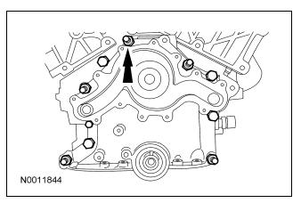
47. Use the special tool to align the front cover and tighten the bolts and stud bolts to 19 Nm (14 lb-ft).
