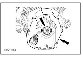
141. **NOTE:** Special bolts are used for flexplate and flywheel installation. Do not use standard bolts.
