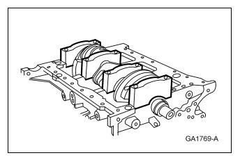
6. Tighten the bolts in the sequence shown to 35 Nm (26 lb-ft) and then rotate an additional 57 degrees.
