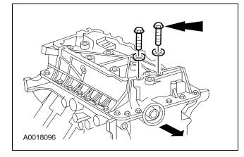
60. Loosely install the 6 remaining lower block cradle bolts.
