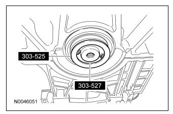
139. Using the special tool, install the crankshaft rear oil seal.
