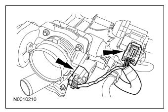
130. Connect the fuel rail pressure and temperature sensor electrical connector and the vacuum tube.
