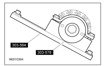
93. NOTE: Camshaft timing slots are off-center.NOTE: Position the camshaft timing slots below centerline of camshaft to correctly fit the
