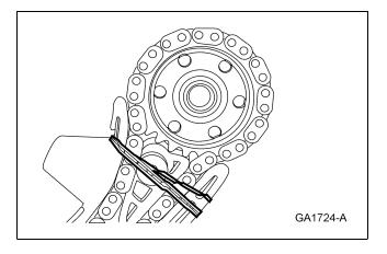
77. CAUTION: The camshaft sprocket must turn freely on the camshaft. DO NOT tighten the bolt.
