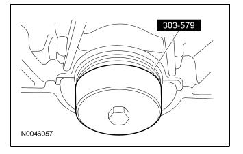
140. Install the spacer plate and if equipped, the flexplate-to-crankshaft spacer.
