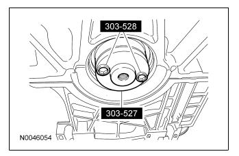
138. Position the crankshaft rear oil seal and the special tool.
