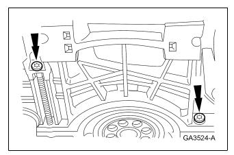
55. **NOTE:** The lower block cradle to the cylinder block alignment must be within a maximum mismatch of 0.25 mm (0.01 in) lower block cradle underflush or 0.05 mm (0.00196 in) lower block cradle protrusion.
