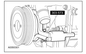
87. NOTE: Camshaft timing slots are off-center.
