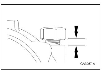
16. Tap on the nut until the bolt can be removed by hand.
