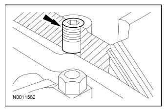
52. Position the lower block cradle and a new gasket.
