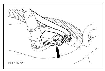
116. Connect the engine coolant temperature (ECT) sensor electrical connector.
