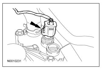
117. Connect the crankshaft position (CKP) sensor electrical connector and attach the 2 wiring retainers.
