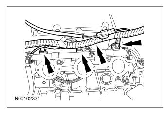
115. Connect the PCV valve electrical connector.
