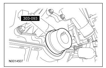
48. **NOTE:** Lubricate the seal lip with clean engine oil.
