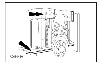
56. Tighten the 20 bolts and the 2 nuts.
