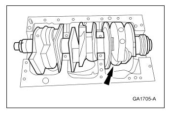
4. **NOTE:** If not secured within 4 minutes, the sealant must be removed and the sealing area cleaned. To clean the sealing area, use silicone gasket remover and metal surface prep. Follow the directions on the packaging. Failure to follow this procedure can cause future oil leakage.
