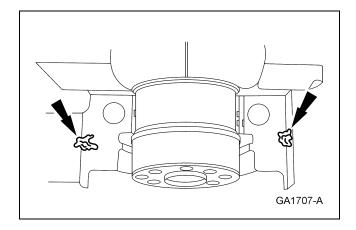
5. Install the main bearing caps in the order in which they were removed.
