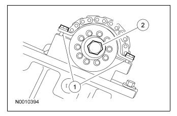
96. Install the LH camshaft tensioner.
