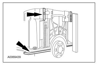
63. Repair all assemblies that exceed underflush specification by installing shims on 1 or both sides of the cylinder block cradle.
