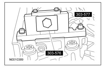
88. **NOTE:** Leave the top 2 special tool clamp bolts loose.
