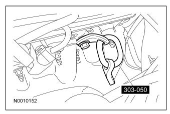
135. Using the special tools, remove the engine from the engine stand.
