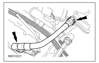
126. Connect the 2 throttle body coolant hoses to the coolant tube.
