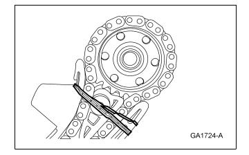
83. CAUTION: The camshaft sprocket must turn freely on the camshaft. DO NOT tighten the bolt.
