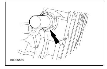
97. Rotate the crankshaft until the cam lobe is in the up position.
