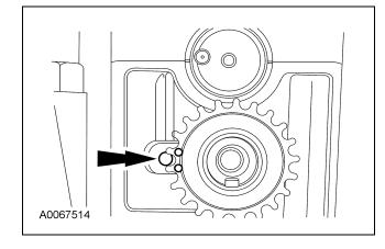
26. If equipped, install the balance shaft chain and crankshaft sprocket.
