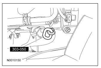
134. Install the special tool to the LH cylinder head.
