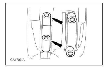
12. **NOTE:** Position the piston with the indentation arrow toward the front of the cylinder block.
