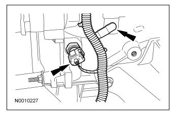
121. Connect the camshaft position (CMP) electrical connector.
