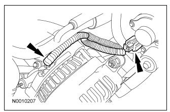
133. Install the special tool to the RH cylinder head.
