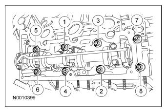
76. Position the RH cassette and camshaft sprocket.
