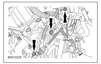
113. Connect the 3 RH fuel injector electrical connectors and attach the wiring retainer to the valve cover stud bolt.
