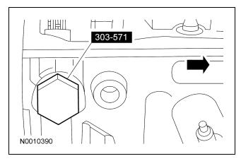
92. **NOTE:** Do not tighten the special tool top 2 clamp bolts. Camshaft sprocket must rotate freely.
