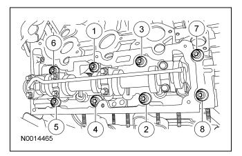
82. Position the LH cassette and camshaft sprocket.
